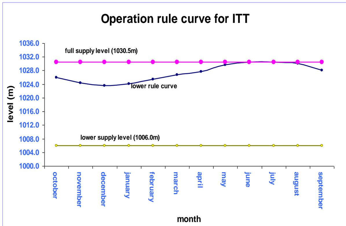
**Figure 1:** Operation Rule Curve for ITT reservoir
